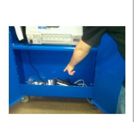
Open the back door of the cart with the barrel key.
